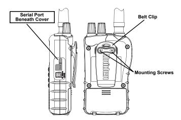
To make your scanner easier to carry when you are on the go, we provide a factory attached belt clip. Use a Phillips screwdriver to remove the mounting screws and the clip from the scanner if desired.
